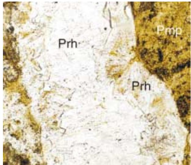
**Photo 5-3.** Photomicrograph showing authigenic mineralogy in the Nakina Formation. The assemblage includes prehnite (Prh) and pumpellyite (Pmp), indicating that these rocks have been subjected to only very low grade metamorphism. Width of the photo represents 1mm.
