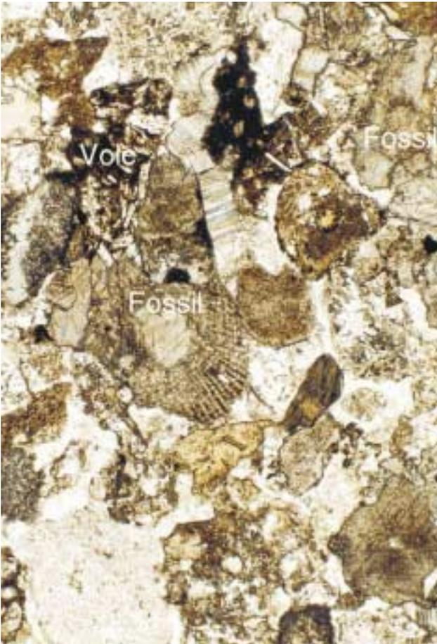
**Photo 5-7.** Photomicrograph of wacke from unit PJs. Long dimension of photo represents 2.5mm.
