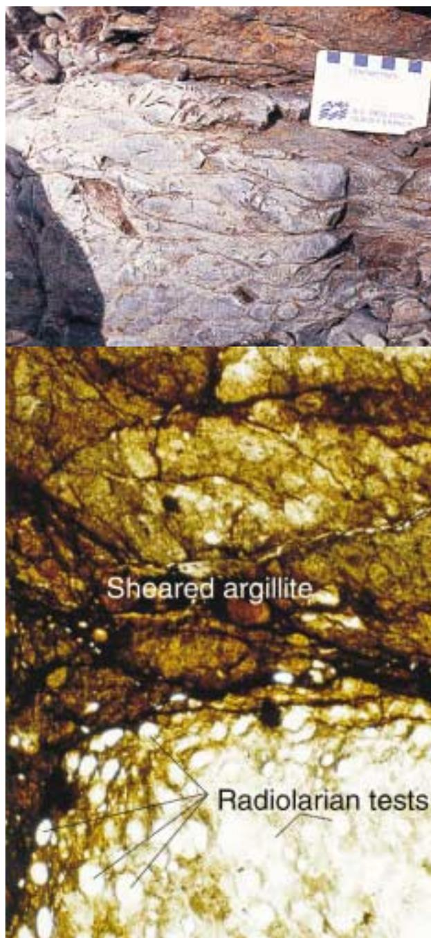
**Photo 5-5.** Broken formation (top) outcrop of disrupted chert layers in an argillite matrix, and (bottom) photomicrograph of radiolarian chert structurally juxtaposed against argillite (long dimension represents 2.5mm).
